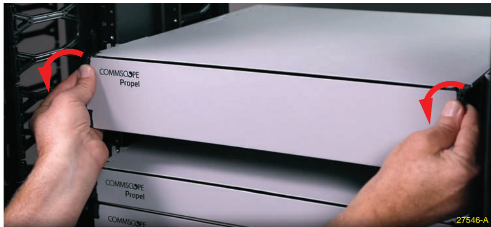
Figure 27. Swinging Down the Front Door of the Propel Fixed Panel
