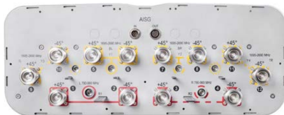
2.4: A base station antenna (BSA) with integrated RET actuators
